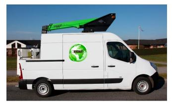
The VERSALIFT 120 mounted on the Renault Master has a working height of 12 meters, a bucketload of 120kg and many other notable features. The VTL-135-FZ has a working height of 13,5 m and the VDTL-140 has a working height of 14 m.
